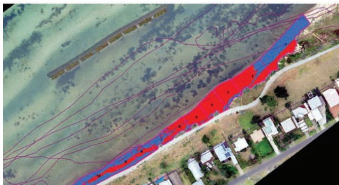
Effects of breakwaters seeded with mussels in retaining sand at Portarlinton, Victoria. (Data from Roob et al. The University of Melbourne/City of Greater Geelong Council).
