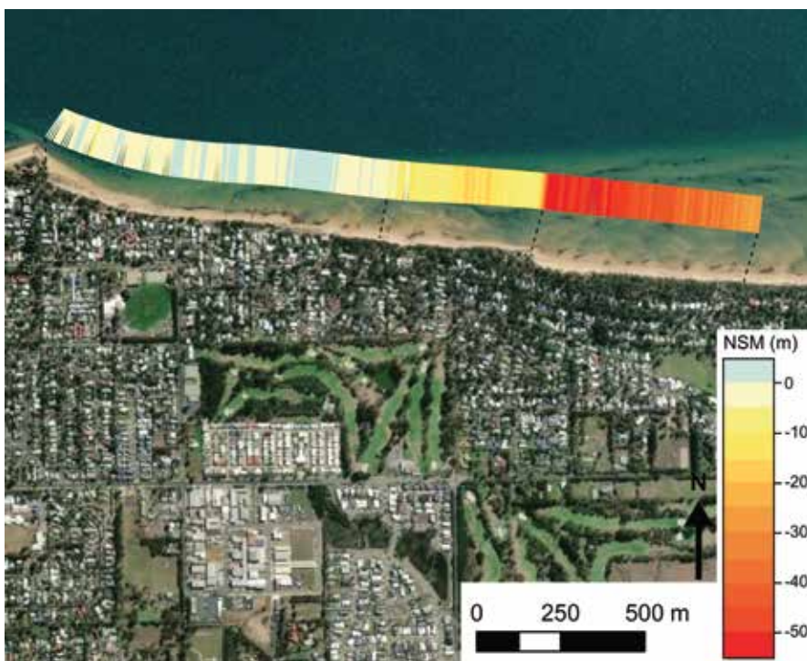
Shoreline change on the Cowes coast showing net shoreline movement (NSM), calculated as the distance between the earliest (1968) and most recent (2019) shorelines. Negative values (yellow/orange/red) indicate landward retreat (erosion) and positive values (green/blue) indicate seaward advance.
